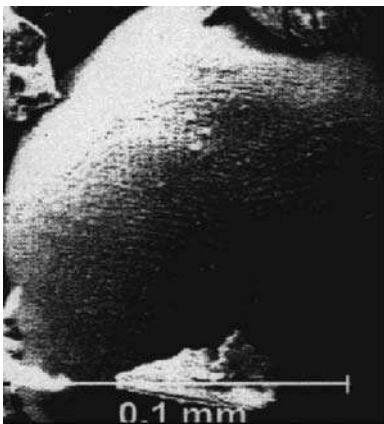
Fig. 2.7. Example of a large grain collected after many discharges in a fusion device [23, 24, 26]
