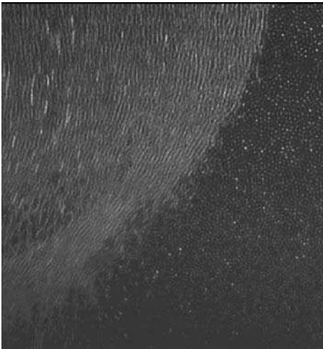
Fig. 1.14. The shear flow excited by an obstacle in the grain flow [79]. The shown region corresponds to the zoomed region in the lower left edge of Fig. 1.12
